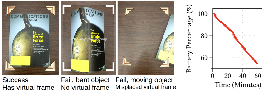
(a) ARCore [44] object detection fails for non-affine transformations. (b) Frequent DNN executions drain battery.
