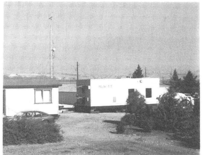
Figure 15. The MoWiTT facility at its field test site in Reno, Nevada. Two sealed insulating glass units are mounted in the two calorimeters. The portable building at left contains the computer that controls the facility and records data, including data from the on-site weather tower. (CBB 8611-10756)
