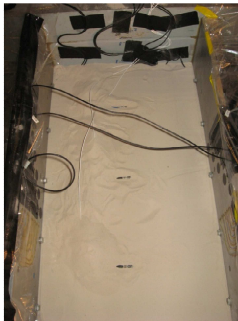
Figure 3.13. Placing accelerometers in the corresponding position.
