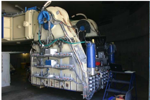
Figure 3.1. The large centrifuge payload bucket at the Center for Geotechnical Modeling at U.C. Davis.
