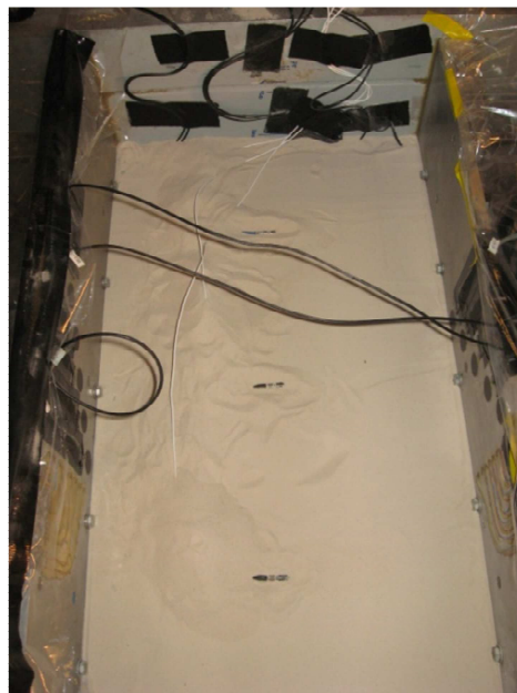
Figure 3.13. Placing accelerometers in the corresponding position.
