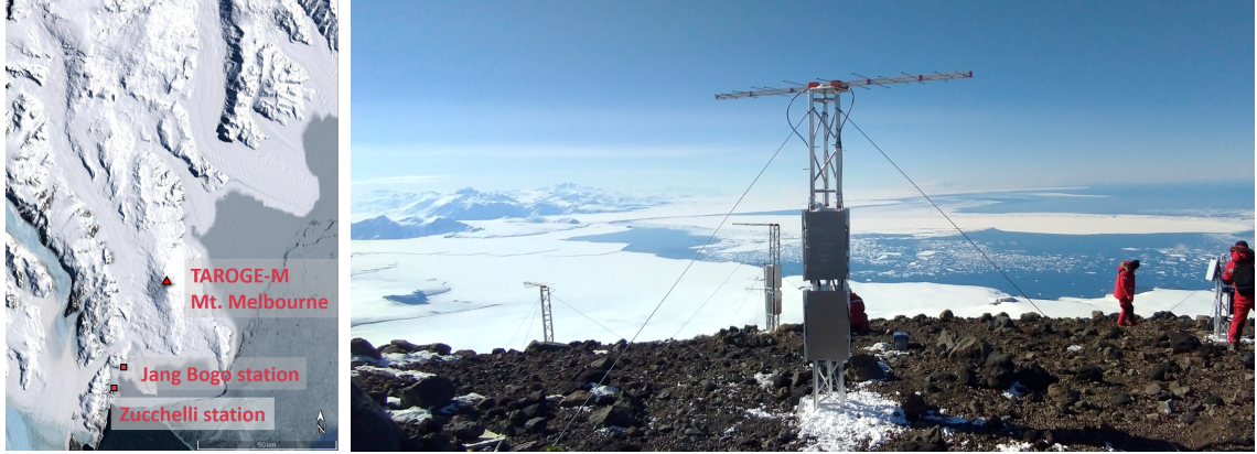
Figure 1. Left: map in the vicinity of Mt. Melbourne (from Google Earth Pro [40]). Right: the first TAROGE-M station atop Mt. Melbourne in Antarctica, deployed in January 2020. Six log-periodic antennas are mounted on 3 m towers, pointing toward the northern horizon (left), with a separation of approximately 8.5 m between the lower three towers, and approximately 19 m between the top (including the veto antenna) and bottom ones, The main DAQ system is placed between the top and the middle towers, whereas the satellite communications antenna and wind turbine are installed on a shorter tower at the back side (right).
