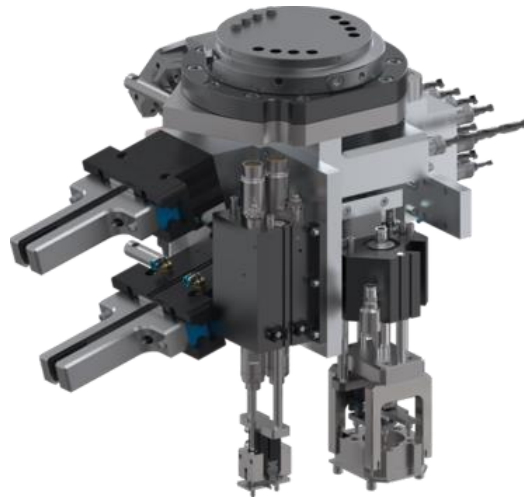
Figure 5 – Example of multi-function head for robotic arm
