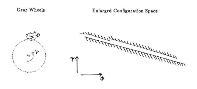
Figure 2: Gear wheels and corresponding configuration space
