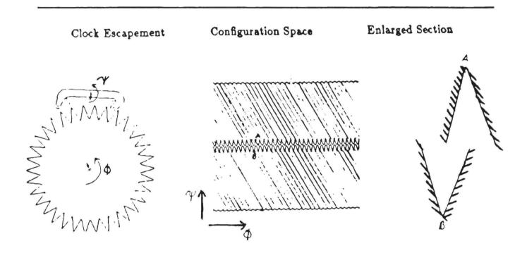
Figure 1: Clock escapement and corresponding configuration space
