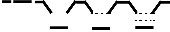
FIG. 3: An array of collectors is shown; from left to right is (a) a flush collector, (b) a recessed collector or capacitive probe, (c) a 1-grid, and (d) a 2-grid collector.
