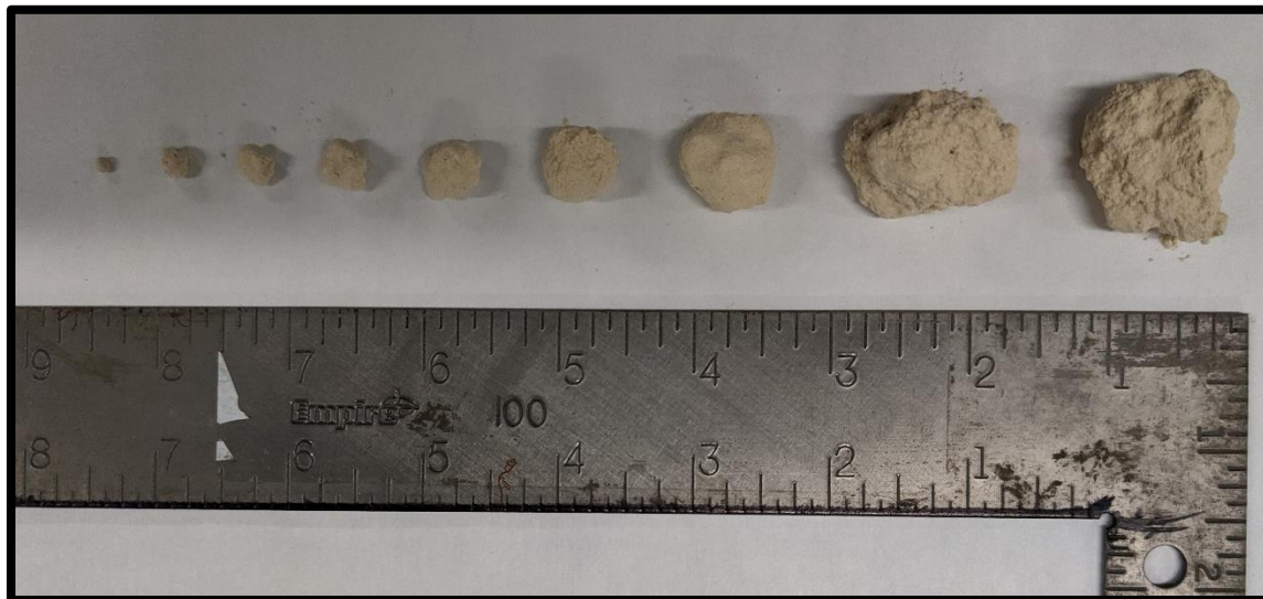
Figure 3: Hydrated nodules in WYFA-2 and WYFA-3, which were sieved before use. WYFA-3 was also heat-treated at 150°C to dehydrate and make it more similar to WYFA-1, which did not have these nodules and had LOI half as large. Scale bar shows inches.
