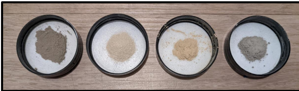
Figure 2: The four SCMs. From left to right: Class C fly ash (FA), paper recycling waste (PW), Wyoming FGD waste ash (WYFA-1), North Dakota fly ash (NDFA)
