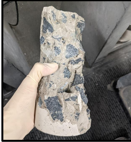
Figure 12: Concrete cylinder (4"×8") after mechanical failure in hydraulic press
