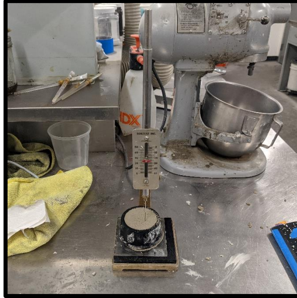
Figure 11: Testing set time of a mortar puck using a Vicat needle apparatus
