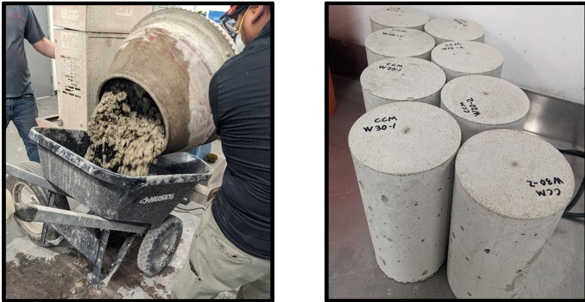
Figure 8: Left: pouring WYFA-3 concrete before it is put into cylindrical molds; Right: 4"×8" concrete cylinders used for mechanical testing
