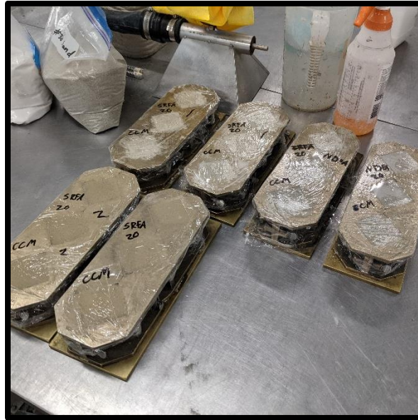
Figure 7: Several mortar cubes in molds after mixing, later used to test compressive strength
