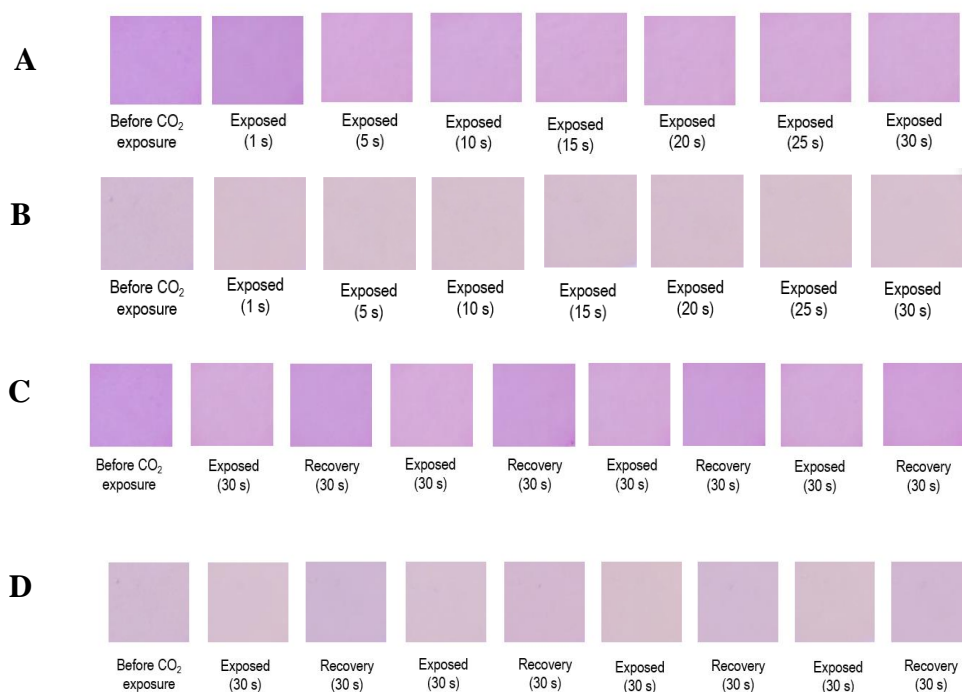
Fig. 3.17 “Colorimetric response time and recovery upon exposure to 2500 ppm CO 2 in humid environment ( 58.8 \pm 3 % RH at 24.7 \pm 0.4 °C). Total flow: 300 sccm. (A) Progression of the color change of PSP-ED/ZIF-8 over 30 s. (B) Progression of the color change of ED/PSP:ZIF-8 over 30 s. (C) Repeat exposure of PSP-ED/ZIF-8 to humid CO 2 . (D) Repeat exposure of ED/PSP:ZIF-8 to humid CO 2 .” Acquired from Davey et al. [123].
