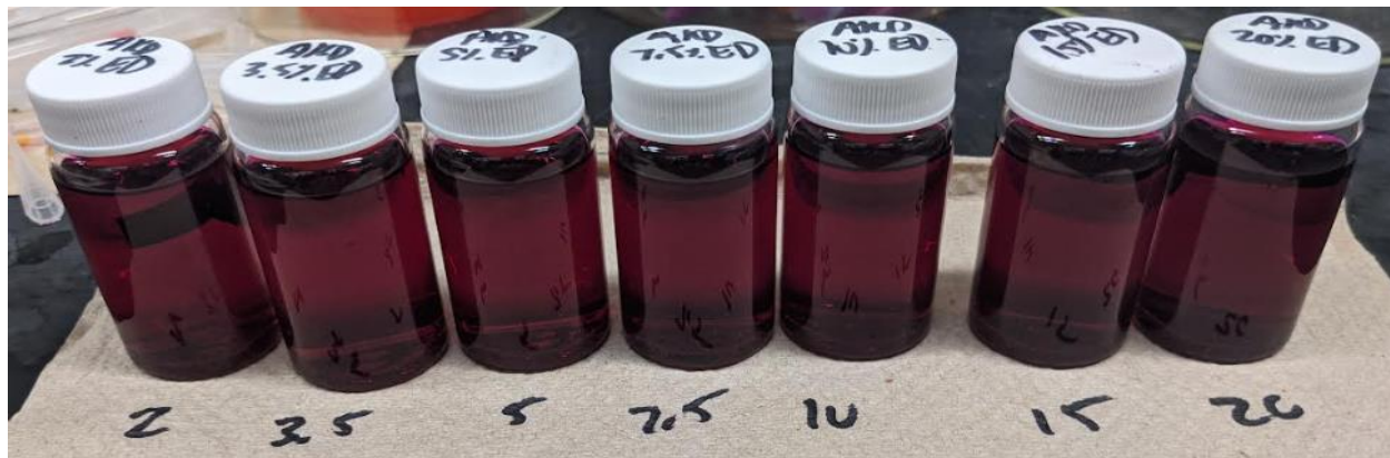
Fig. 4.19. Ethylenediamine solutions (up to 20%, % v/v in methanol). Dye loadings are set constant at 0.5 mg phenol red/ml solvent.
