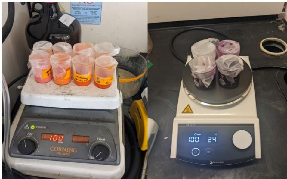
Fig. 4.17. Room-temperature equilibrium mixing of pristine ZIF-8 with (A) phenol red in methanol and (B) phenol red in a 2% ethylenediamine methanolic solution.
