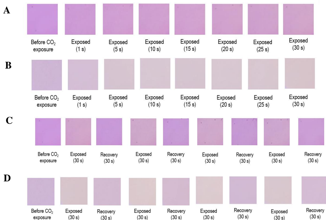
Fig. 3.16 “Colorimetric response time and recovery upon exposure to 2500 ppm CO 2 in humid environment ( 34.6 \pm 3 % RH at 24.7 \pm 0.4 °C). Total flow: 300 sccm. (A) Progression of the color change of PSP-ED/ZIF-8 over 30 s. (B) Progression of the color change of ED/PSP:ZIF-8 over 30 s. (C) Repeat exposure of PSP-ED/ZIF-8 to humid CO 2 . (D) Repeat exposure of ED/PSP:ZIF-8 to humid CO 2 .” Acquired from Davey et al. [123].
