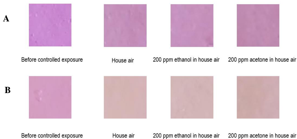
Fig. 3.21 “Colorimetric exposure to dry house air, dry house air mixed with 200 ppm ethanol, and dry house air mixed with 200 ppm acetone. Row A: PSP-ED/ZIF-8 (first-generation material). Row B: ED/PSP:ZIF-8 (second-generation material). Dry house air is 458 \pm 3 ppm CO 2 .” Acquired from Davey et al. [123].
