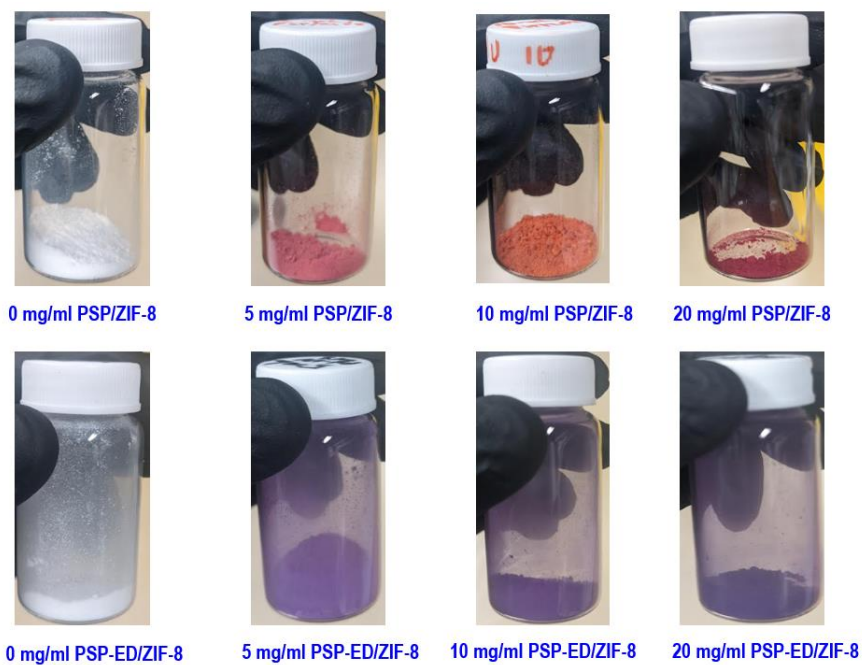
Fig. 4.18. (Top row): PSP/ZIF-8 powders (0% ethylenediamine in methanol). (Bottom row): PSP-ED/ZIF-8 (2% ethylenediamine in methanol). Concentrations are shown in mg/ml phenol red (in either methanol or ethylenediamine/methanol solution).
