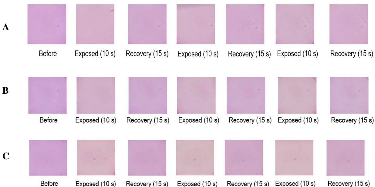
Fig. 2.19. “Effect of repeated exposure of PSP-ED/ZIF-8 to (A) 700 ppm CO 2 , (B) 3,000 ppm CO 2 and (C) 7,500 ppm CO 2 in dry atmosphere.” Acquired from Davey et al. (2021). [99].
