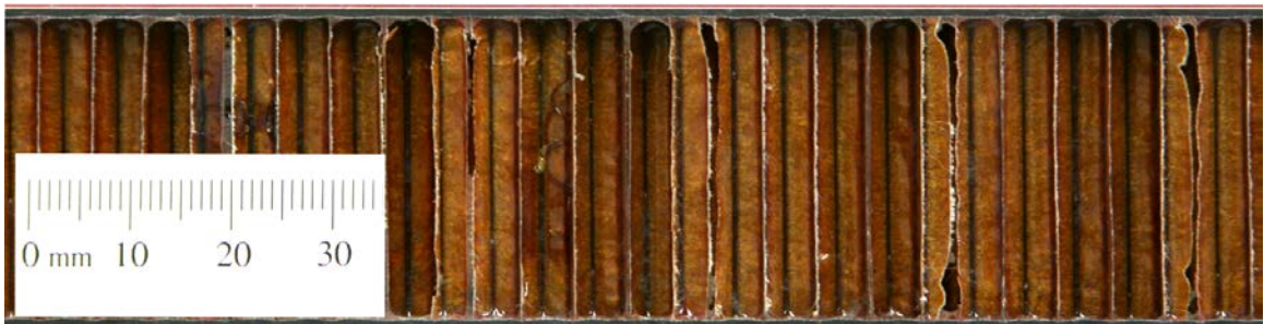
Peak dent 0.02 mm, Test-032 on thick facesheet Panel A05 (49.38 m/s at 25 degrees), ice broke prior to impact, very slightly noticeable dent, minor Mode I core wrinkle
