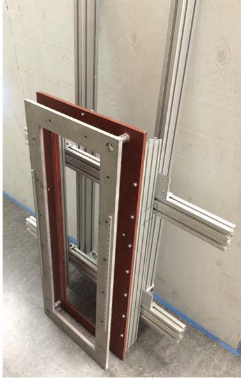
Figure 2.4.2. Panel-Holding Test Fixture.
