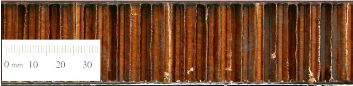
Peak dent 0, Test-045 on thick facesheet Panel A07 (speed unknown at 40 degrees), ice crushed before impact, no visible dent, no core damage
