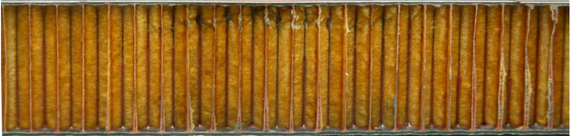
Peak dent 0.53 mm, Test-005 on thin facesheet Panel A05 (23.67 m/s at 40 degrees), visible dent with Mode II core buckling
