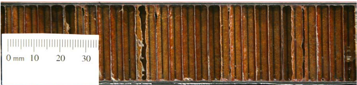
Peak dent 0.04 mm, Test-008 on thin facesheet Panel A03 (23.90 m/s at 25 degrees), no visible dent with Mode I core wrinkling
