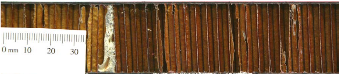
Peak dent 0.07 mm, Test-017 on thin facesheet Panel A04 (28.02 m/s at 25 degrees), no visible dent with Mode I core wrinkling
