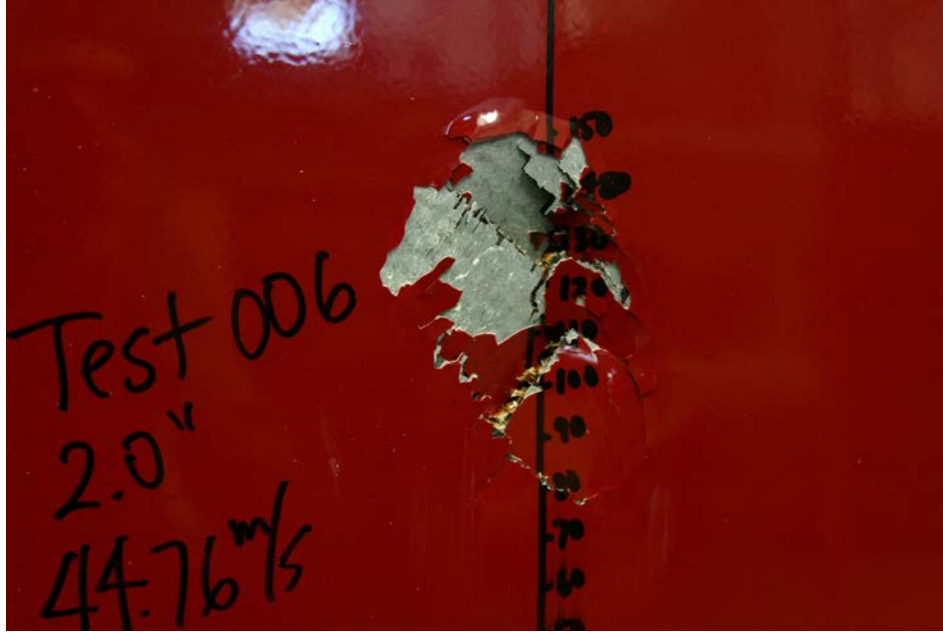
Figure 3.2.5. Visible skin penetration from Test-006 on thin facesheet Panel A02 (40 degrees).
