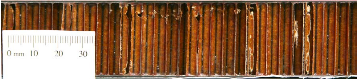
Peak dent 0.35 mm, Test-018 on thick facesheet Panel A04 (48.26 m/s at 25 degrees), ice cracked, slid and then reflected off the panel, visible dent with Mode III core fracture
