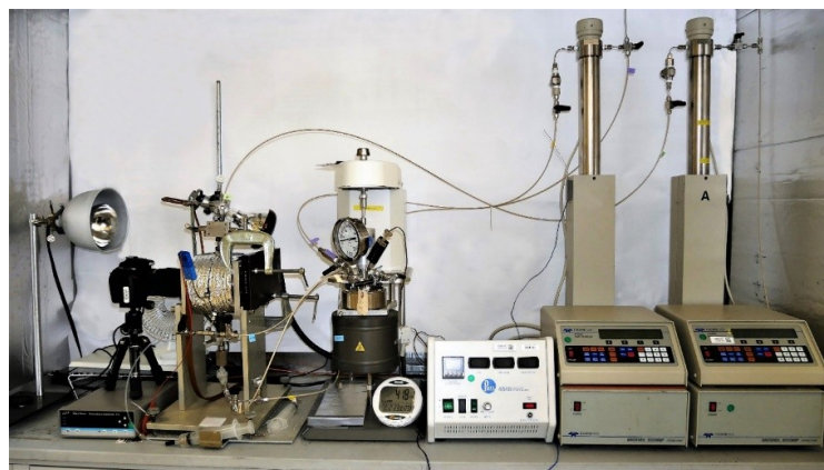
196 Figure 3 Schematic diagram of the experimental systems and photographs of the 197 experimental setup for contact angle measurements.
