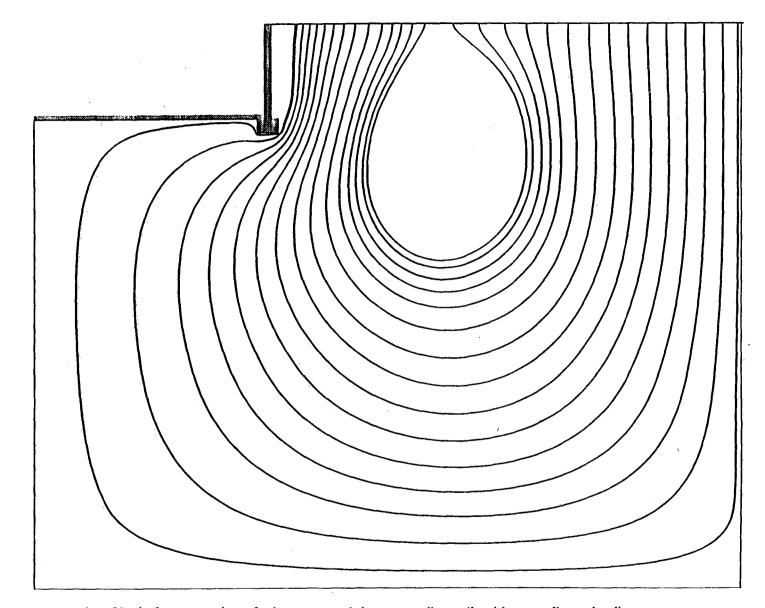
4. Vertical cross-section of a basement and the surrounding soil, with streamlines; the direction of flow is clockwise. In this case there is no pressure difference between basement and outside, so that the flow is a circulation due to natural convection. The temperatures of the basement, the soil surface, and the lower soil boundary are 15, 0, and 10 °C, respectively.
