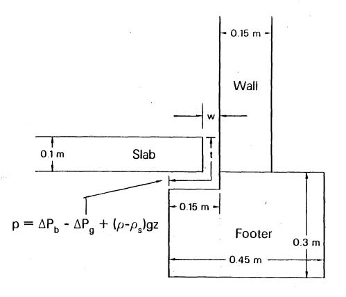
Vertical surfaces:  $T = T_b$ ;  $\frac{\partial p}{\partial r} = 0$ ;  $\frac{\partial C}{\partial r} = 0$ Horizontal surfaces:  $T = T_b$ ;  $\frac{\partial p}{\partial z} = (\rho - \rho_s)g$ ;  $\frac{\partial C}{\partial z} = 0$
