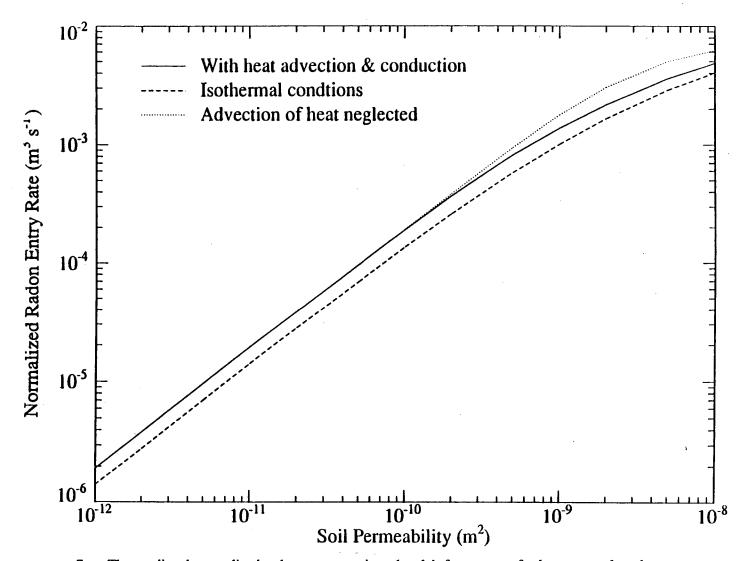
7. The predicted normalized radon entry rate into the slab-footer gap of a basement, plotted against soil permeability, for the configuration of Figures 1 and 2. The basement is 5 Pa below atmospheric pressure. The solid line shows the predicted rates when both thermal conduction and convection are included in the model. The basement, outside, and deep soil temperatures are 15, 0, and 10 °C, respectively. The dashed line shows the predictions when thermal convection is neglected.
