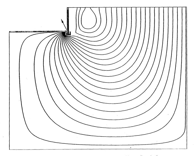
6. Vertical cross-section of a basement and the surrounding soil, with streamlines; the direction of flow is clockwise. In this case both forced and natural convection are present. The basement pressure is 5 Pa below that of the atmosphere. The temperatures of the basement, the soil surface, and the lower soil boundary are 15, 0, and 10 C, respectively.
