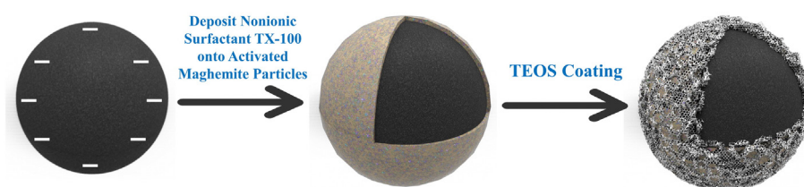
Fig. 1. Schematic representation of Mag-PCMA-T synthesis (note: the core and shell are not drawn to scale).
