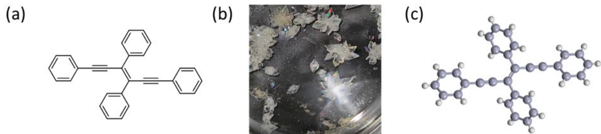
Figure 15. Crystal structure of tetraphenyl trans -3-hexene-1,5-diyne (TPE). (a) TPE; (b) white crystals obtained by slow evaporation of chloroform; (c) Representation of the crystal structure using Cambridge Crystallographic Database software called Mercury.
