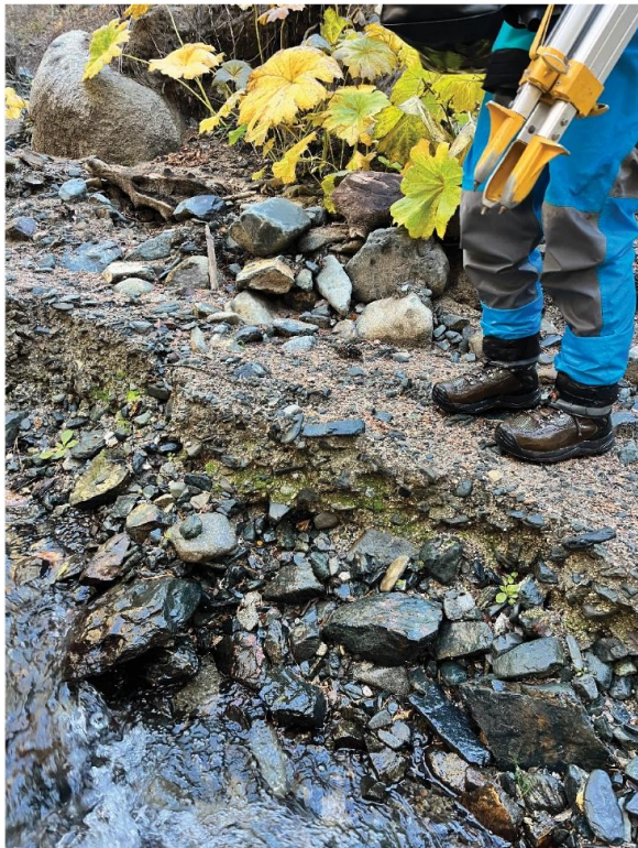
Figure 7c. The channel is made of noncohesive sediments suggesting high rates of bed material transport throughout the incised channel. View of left bank (looking downstream).
