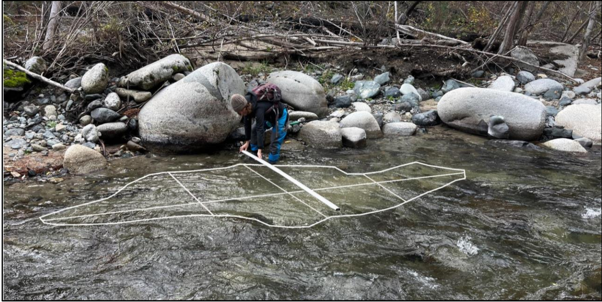
Figure 6. Example of measurements taken for each bar (image of bar 2). The 3 width measurements were averaged and multiplied by the length to determine area estimates.
