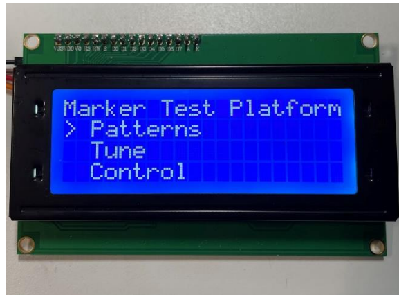
Figure 10: This is the main menu used to control the Arduino and XYZ Platform.
