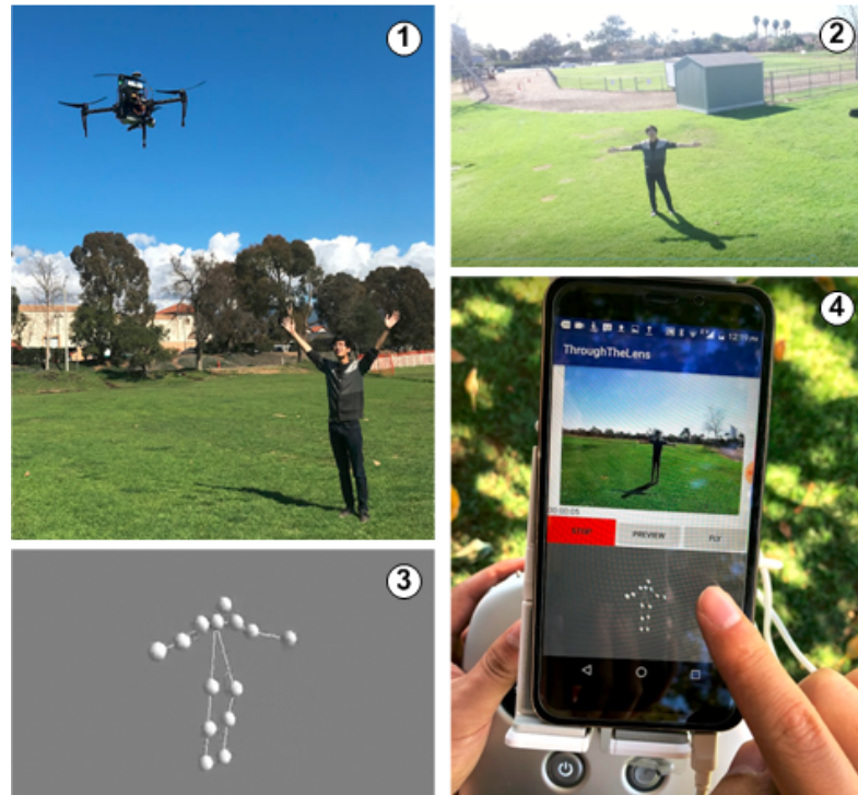
Figure 3.14: Overview of the through-the-lens drone filming. (1) The filming scene. (2) Camera View. (3) The preview of 3D human model estimated from camera view. (4) User manipulates the 3D model in the preview to design the viewpoint.
