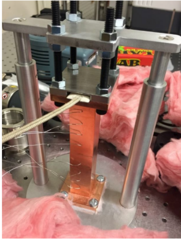
Figure B.2: Image of cut-bar experimental setup used to determine the thermal conductivities of the samples described above.
