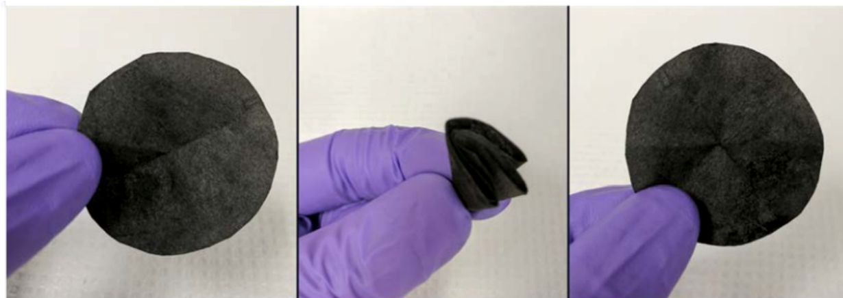
Figure A.3: Folding and unfolding of the GO leaf to demonstrate its material durability.
