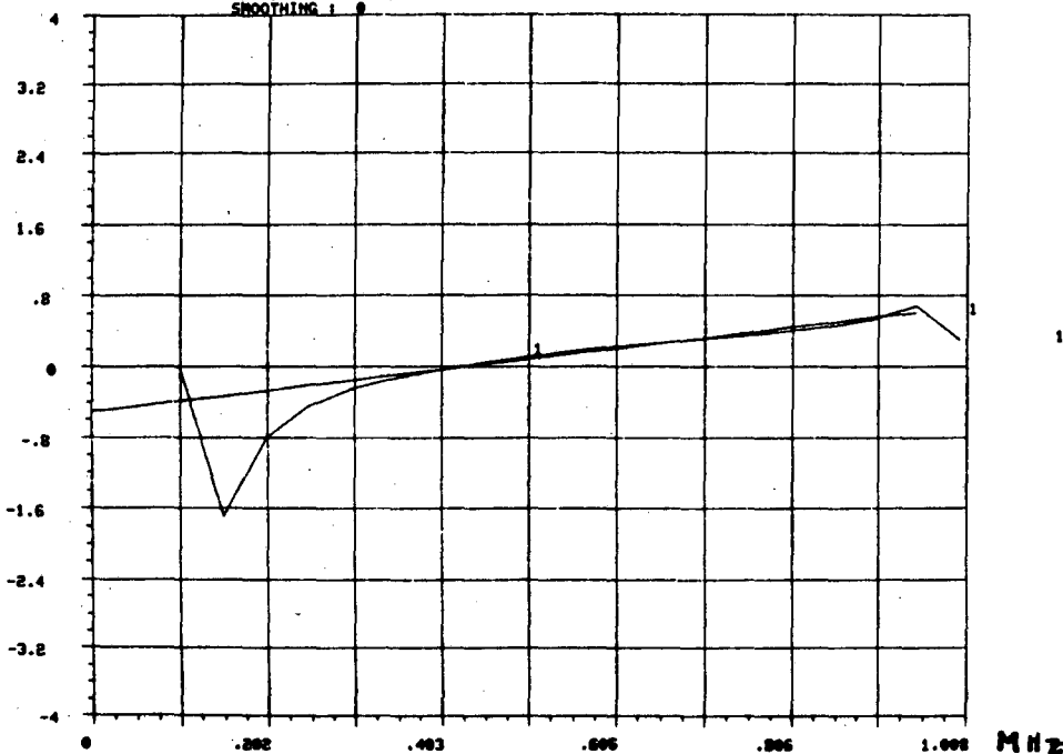
Fig. 7.16 Spectral ratio between the spectra from the aluminum standard and the 7.622 cm long perspex specimen.
