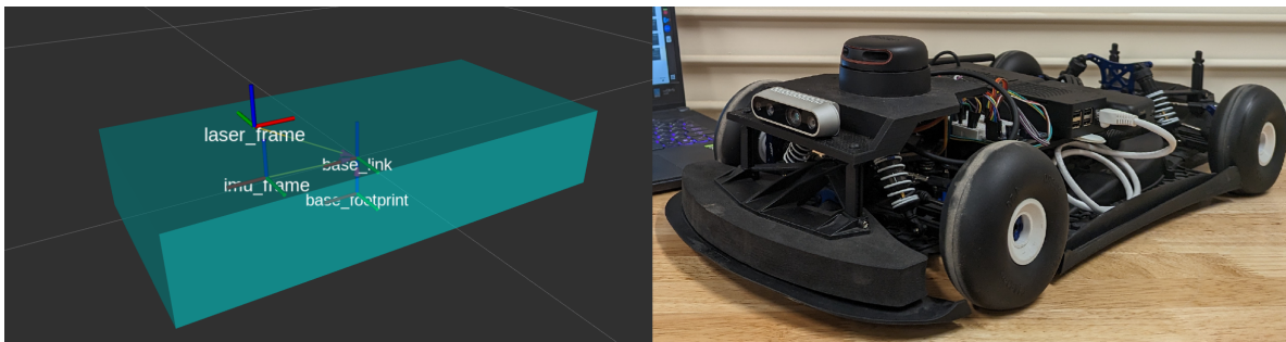
Figure 3.6: Coordinate Frames Provided in ROS, Compared to Physical Car
