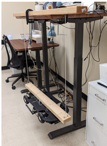
Figure 3.2: Bifilar Pendulum with Scale Car Mounted, for Moment of Inertia Calculations
