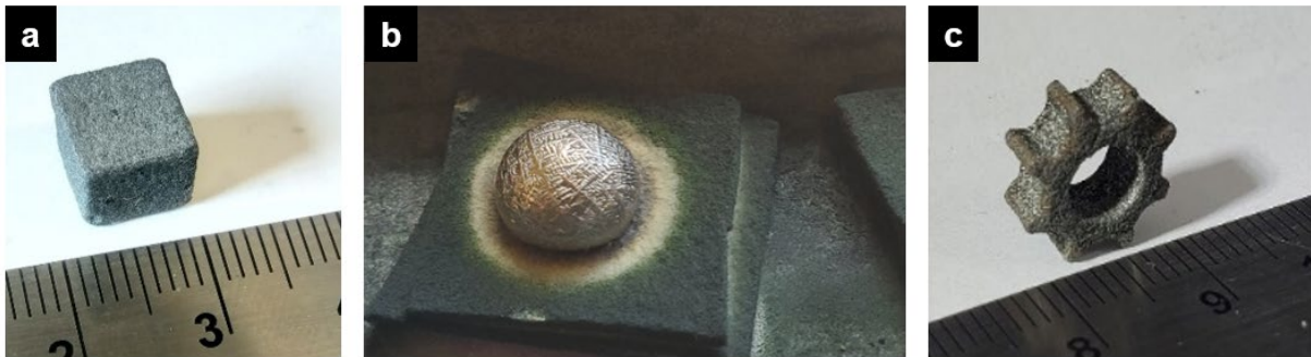
Figure 3.8 Sintered SS316L after SJ and debinding (a) 99% SS316L cube, (b) 90% SS316L cube and (c) gear
