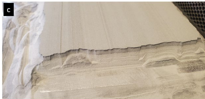
Figure 4.28 Schematic describing the SLM setup for the processing of functionally graded SS316L-WC (a) at start of printing (b) at the end of printing (c) actual powder bed in the build platform after sample removal
