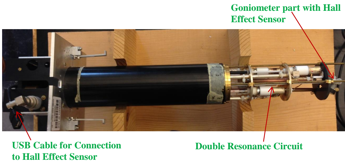
Figure 2.13 Overview of the single-crystal probe (without ground shell)
