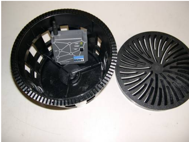
Figure 9: Mote deployed in diffuser
