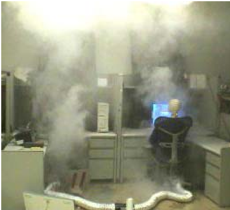
Figure 94: Side-by-side comparison of plumes generated by artificial loads (left) and real workstation loads (right), using smoke for visualization.
