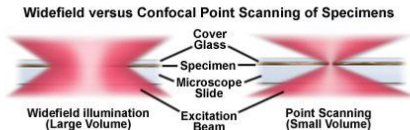
Figure 37 Typical specimen illumination utilized by Wide-field vs. Confocal Microscopy 154
