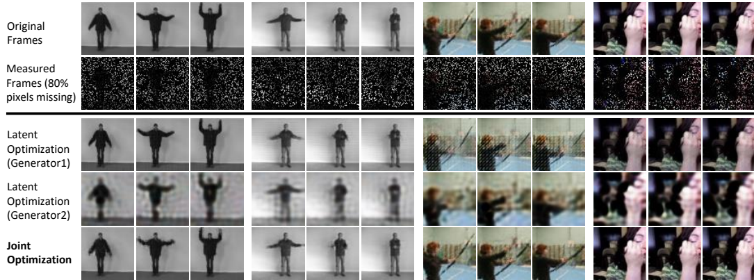
Figure 4.3: Joint optimization versus latent code optimization. First row is the true images of the videos sequences. The second row contains the masked samples of the sequences. In the third row, we reconstruct frames with latent code optimization using a generator trained on some other frames of the same video sequence (Generator1). In the fourth row, we use latent code optimization with a generator trained on CIFAR10 dataset (Generator2). The fourth row is the reconstruction with joint optimization of generator initialized with random weights. We can observe that latent code optimization does not perform well (row 4) when we do not have generator pretrained on similar distribution. However, joint optimization performs as good as as or better than latent code optimization without any pretrained weights.
