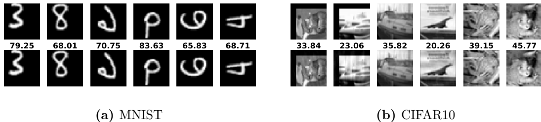
Figure 9.4: Test results on shifted/flipped/rotated images using the reference learned on upright-centered (canonical) images. PSNR shown on top of images.
