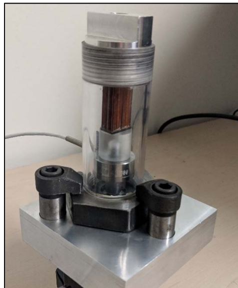
Figure 3.65. In-situ load frame
