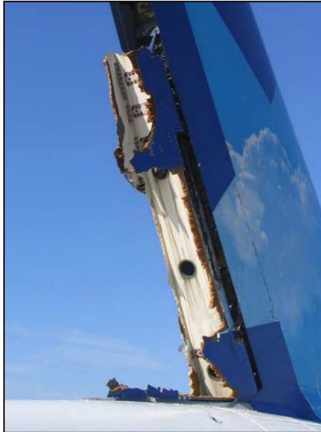
Figure 1.12. Side view of vertical tail plane and residuals of rudder of Airbus A310-308 aircraft after Air Transat Flight 961 [Transportation Safety Board of Canada, 2005]
