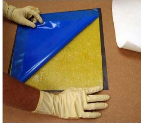
d) Applying film adhesive
