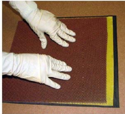
e) Inserting honeycomb core
