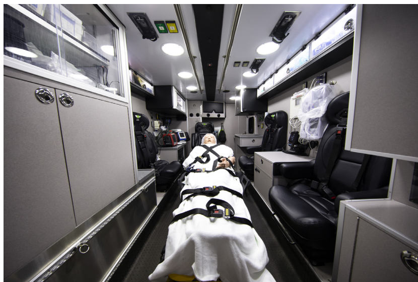
Figure 2. Critical care transport vehicles like Parkview Health's MICU Ford F-550 with an Osage Ambulance Super Warrior "68" box have the capacity to hold up to 4 caregivers in the patient care area, along with multiple pieces of equipment, medications, and supplies to maintain the high level of care provided in the ICU. This MICU has a liquid oxygen system that holds 5 to 6 times more oxygen than a standard ground ambulance. (Courtesy of Ryne Hastings, Parkview Health.)
