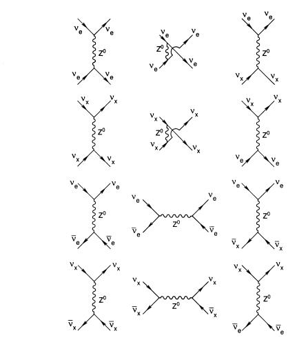
FIG. 2.—Feynman diagrams involving the weak neutral current that contributes to the effective mass of neutrinos in a background plasma. Contributions from neutral current interactions on the charged leptons are neglected since they are identical for each neutrino flavor.
