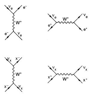
FIG. 1.—Feynman diagrams involving the weak charged current that contributes to the effective mass of neutrinos in a background plasma.
