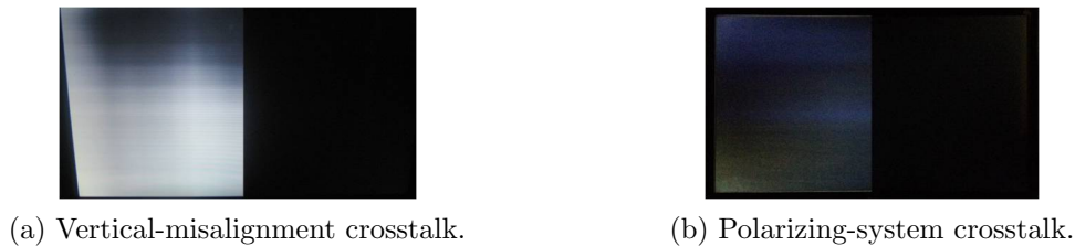
Figure 4.2: Comparison of VM-based crosstalk and the crosstalk induced by the polarizing system, where the level of crosstalk is indicated by the brightness of the screen on the left half.
