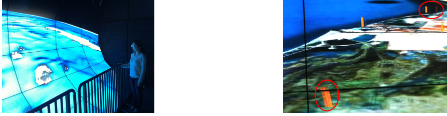
Figure 3.2: Crosstalk in passive-type circularly polarized LCD. Left: Immersive 3D formed by the CPLCD grid. Right: Crosstalk in the CPLCD grid.
