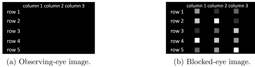
Figure 4.10: Subjective test on crosstalk caused by vertical misalignment (VM) of light in CP LCD. (a) and (b) are input images.
