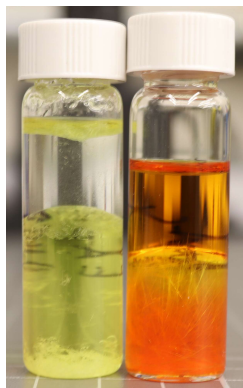
Figure 3.11. Reaction of EAcAc (left) and AcAc (right) with 1 wt % HMTA in DI water. Color and precipitates are the results of undesirable side reactions occurring between HMTA (gelling agent) and EAcAc/AcAc (chelating agent).
