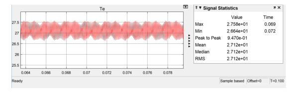
Figure 28 The result of torque after adding harmonics based on nearest three vectors method (m=0.36)
