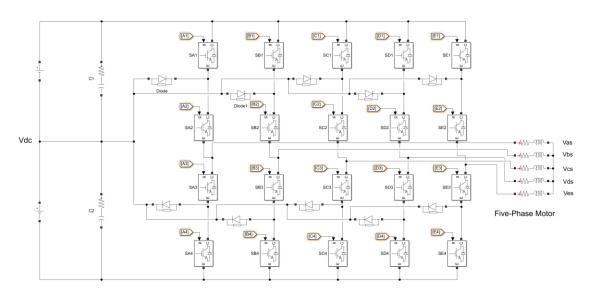
Figure 1. The scheme of three-level five-phase VSI
