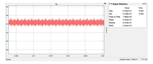
Figure 26 The result of torque after adding harmonics based on nearest three vectors method (m=0.54)
