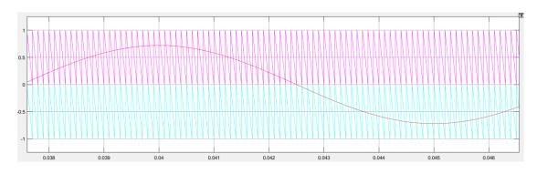
Figure 20. Three-level sine- triangle modulation
