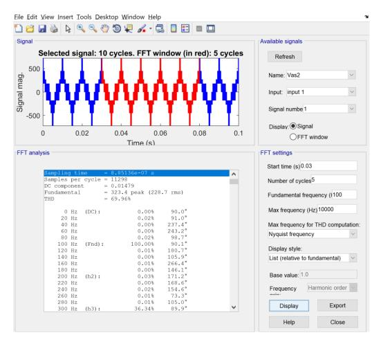
Figure 24 FFT analysis of phase voltage by using nearest three vectors method (m=0.36)
