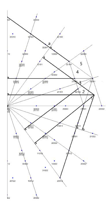
Figure 9. Switching sequences selector and region determination with high modulation index
