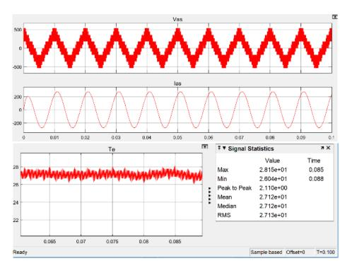
Figure 17. Simulated motor phase voltage, current and torque by using optimized method with low m
