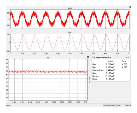
Figure 14. Simulated motor phase voltage, current and torque by using nearest three vectors with high m
