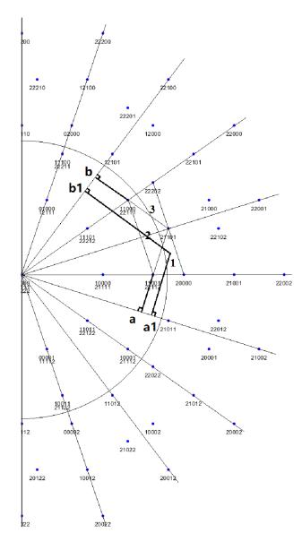
Figure 8. Switching sequences selector and region determination with low modulation index
