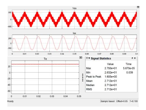
Figure 22 Simulated motor phase voltage, current and torque by using sine-triangle method with low m
