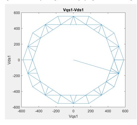
Figure 15. Vds1-Vqs1 plot by using nearest three vectors with high m
