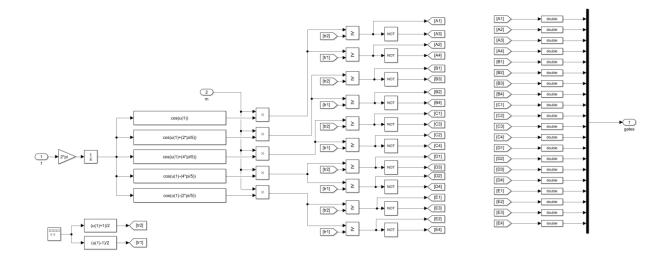
Figure 21. Three-level sine- triangle implementation in MATLAB/Simulink
