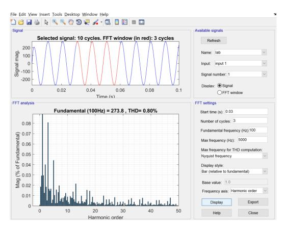
Figure 19 FFT analysis by using optimized method with low m
