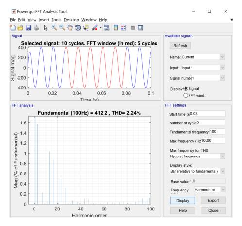
Figure 16 FFT analysis by using nearest three vectors with high m
