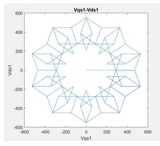
Figure 29 Vds1-Vqs1 plot of harmonics injection (m=0.36)
