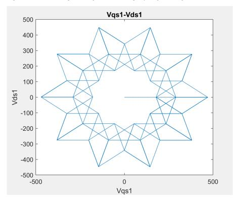
Figure 23 Vds1-Vqs1 plot by using sine-triangle method with low m
