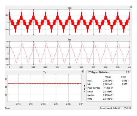
Figure 11. Simulated motor phase voltage, current and torque by using nearest three vectors with low m
