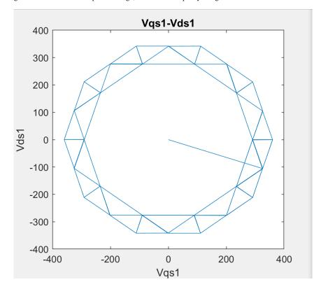
Figure 12. Vds1-Vqs1 plot by using nearest three vectors with low m
