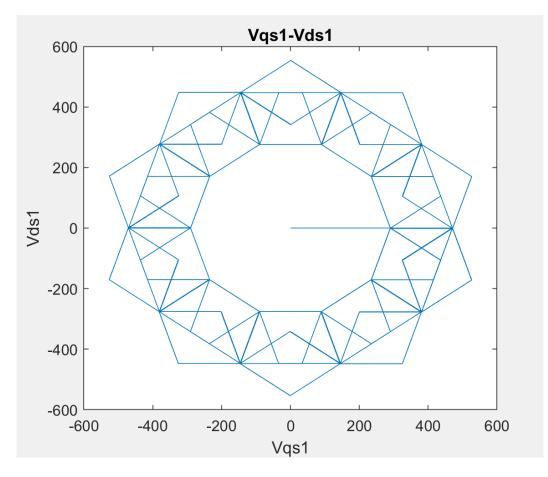
Figure 27 Vds1-Vqs1 plot of harmonics injection (m=0.54)
