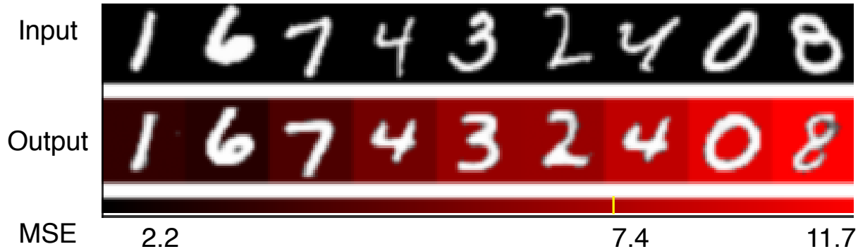
Figure 1: Limitation of novelty detection using image reconstruction error. Top: Input images. Middle: Output images of adversarial autoencoder (AAE). Bottom: mean squared error (MSE) of all images. We set the images of digits of 0-8 and 9 as normal and novelty, respectively. Since mean of novelty scores among the image of digit 9 (novelty class) is 7.4, MSE values of normal image bigger than 7.4 lead to wrong novelty detection.
