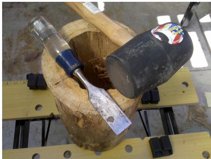
Figure 2.1: Boring through the eucalyptus tree trunk.
