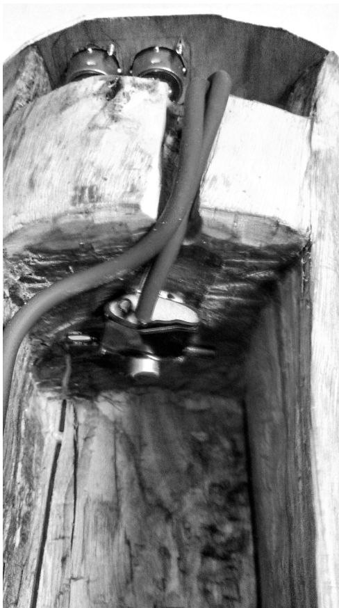
Figure 3.10: Microphones mounted on the teponaztli.
