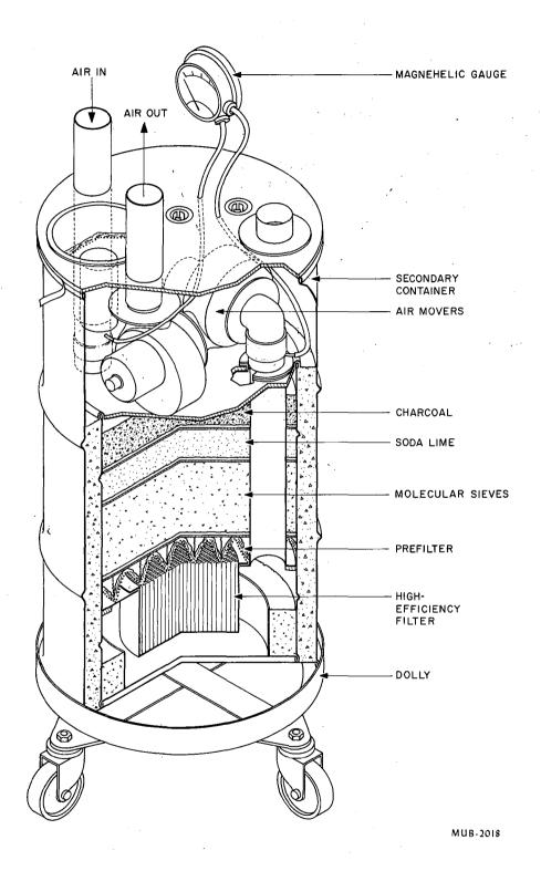
Fig. 1. Cutaway drawing of dry-scrubber unit.
