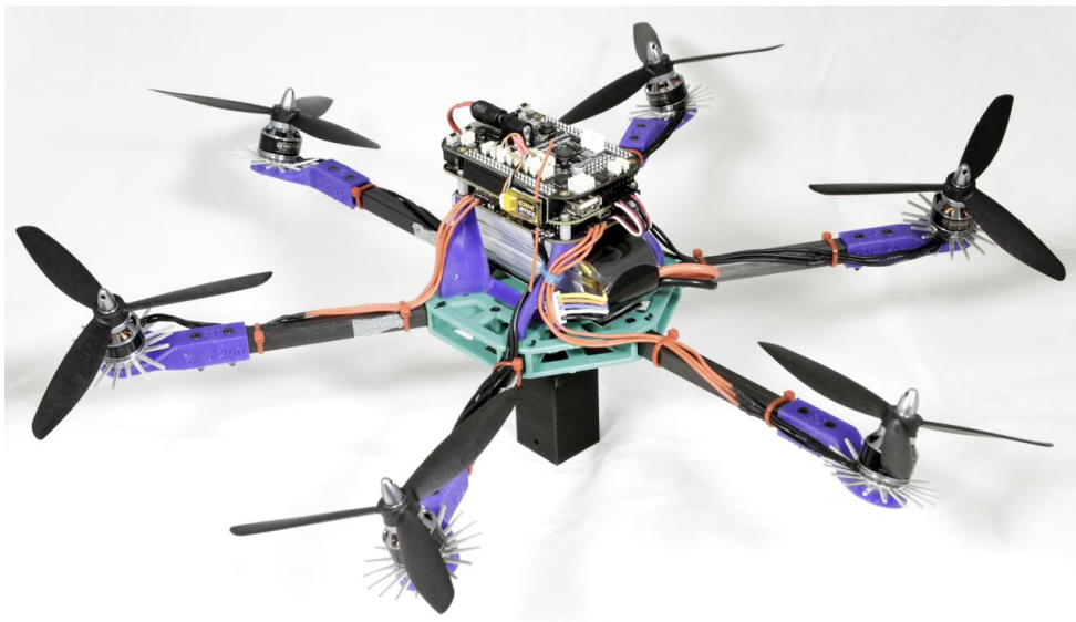
Figure 5.4: Isometric view of case study airframe highlighting the rotor angles.
