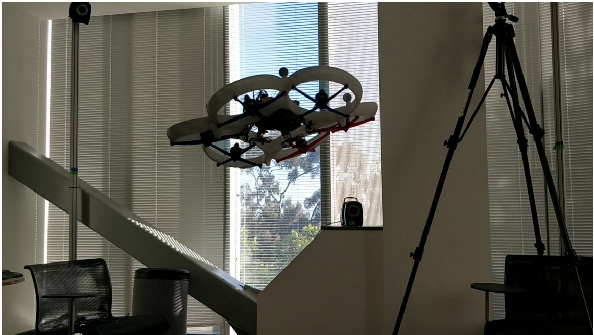
Figure 5.3: EduMAV in flight inside Vicon Motion Capture System.
