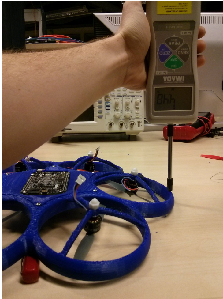
Figure 4.9: Prototype 3D printed model undergoing static stiffness validation.
