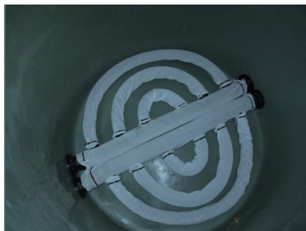
Fig. 1. Drainage pipes and a filter sock placed at the bottom of the lysimeter.
