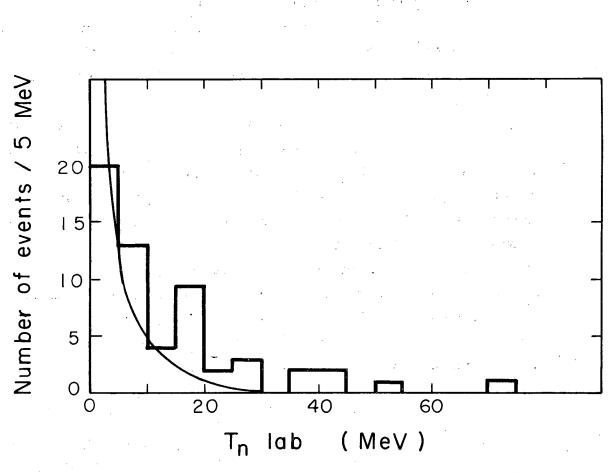
Fig. 16. Histogram of the laboratory-system kinetic energy of the neutron in the reaction  $K^- + d \rightarrow \Sigma^- + \pi^+ + n$ . The curve is the prediction according to the impulse model.
