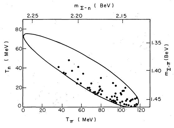
Fig. 12. Normalized Dalitz plot for the reaction  $K^- + d \rightarrow \Sigma^+ + \pi^- + n$ .
