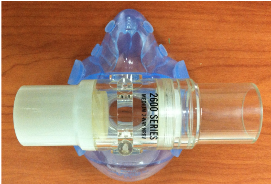
Figure 3.2: Breathing Mask (7400 series Oro-Nasal Mask, Hans Rudolph) + Two-way non-rebreathing valve (2600 Medium). The breathing line setup is divided into three major parts, Mask, Inspiratory Line and Expiratory Line. The human subject wears a breathing mask in the MR bore. Inspiratory equipment is in the MR scanner room. Expiratory gas is displaced to a metabolic cart system in MR console room through expiratory line.
