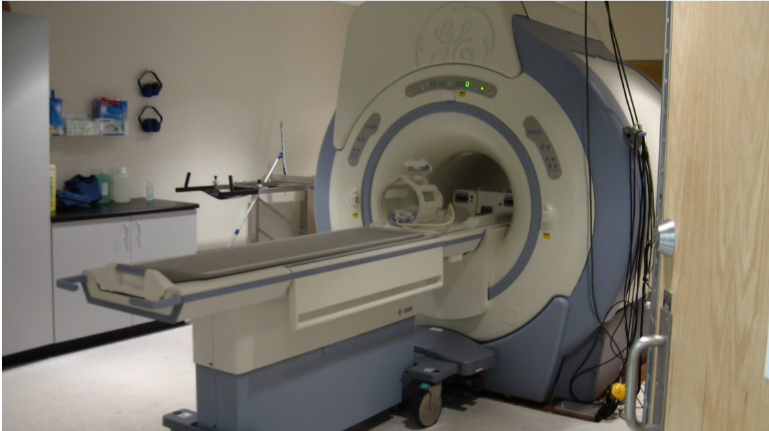
Figure 2.1: MRI Scanner at UCSD Radiology Imaging Laboratory (1.5 T GE HDx EXICITE twinspeed scanner, GE Healthcare). http://ril.ucsd.edu/
