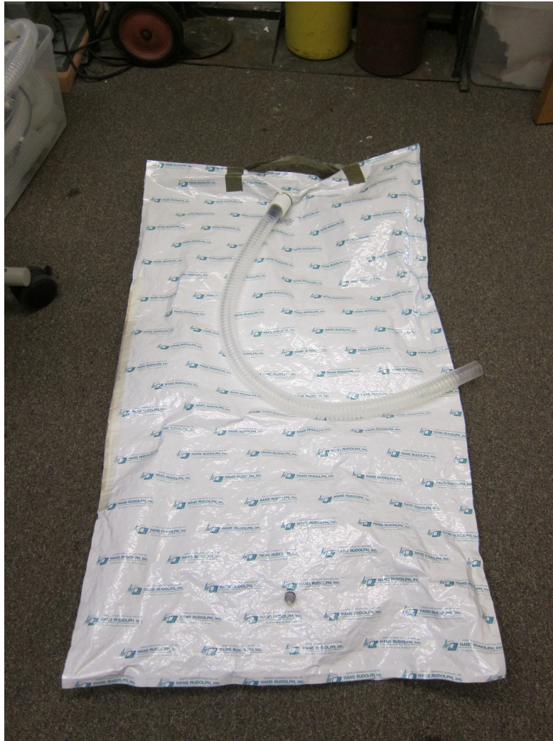
Figure 3.4: Mylar gas bag (Non-diffusing gas collection bag 170 liter, Hans Rudolph). One end of the switching valve was connected to an inspiratory Mylar gas. For a study involving different inspiratory oxygen concentrations, a 170-liter Mylar bag was used to hold either hyperoxic or hypoxic gas mixtures [1, 2].
