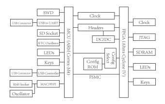
Figure 11: Original system organization of the ARM-FPGA hybrid system.
