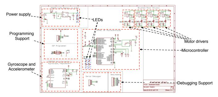
Figure 2: This schematic for a remote controlled "quadcopter" illustrates how traditional schematics excel at describing the structure of as circuit. However, they cannot express complex relationships between components or break the circuit into independent, parameterizable modules.
