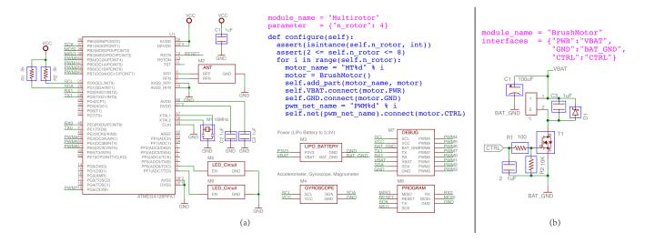
Figure 9: In the Echidna schematic for configurable multirotor aircraft, the top-level module (a) instantiates n\_rotor copies of the BrushMotor module (b). The whole design contains over 60 discrete components, but only a fraction are visible at the top level, providing a clearer picture of the circuit's structure.
