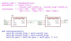
Figure 6: Example schematic of combining a low-pass filter and a high-pass filter to get a band-pass filter.
