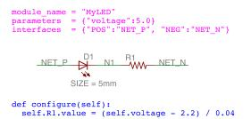
Figure 3: Echidna allows the designer to parameterized circuits and define relationships between components. In this case, the code in blue sets the resistance of R1 based on the voltage parameter.
