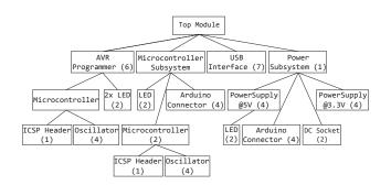
Figure 10: Breaking the design of the Arduino Uno into Echidna modules hides many details of the design from the top-level. The number in parenthesis indicates number of terminal submodules inside the corresponding module.
