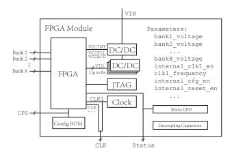
Figure 13: The FPGA module. We embed common supporting circuit of FPGA inside a wrapper and use parameters to customize them. This FPGA module hides trivial but necessary circuit from its user. It has much clearer interfaces, and is reusable in various designs.
