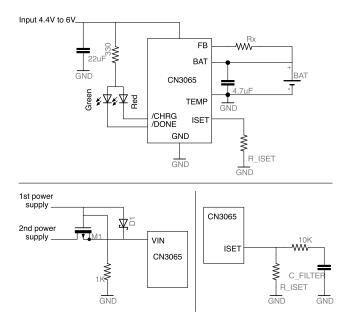
Figure 1: The reference schematics from the datasheet for a lithium polymer battery charger [3] provide only partial documentation for configuring the device and leave the designer to perform tedious and error-prone calculations.
