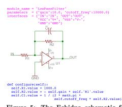
Figure 5: The Echidna schematic for a firstorder, low-pass filter uses Python code to calculate circuit values based on the gain and freq parameters.
