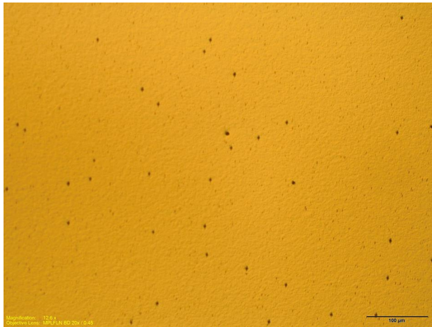
Figure 4.16. Optical microscope of the surface of 1.3 \mu\text{m} of InGaP grown on GoVS.
