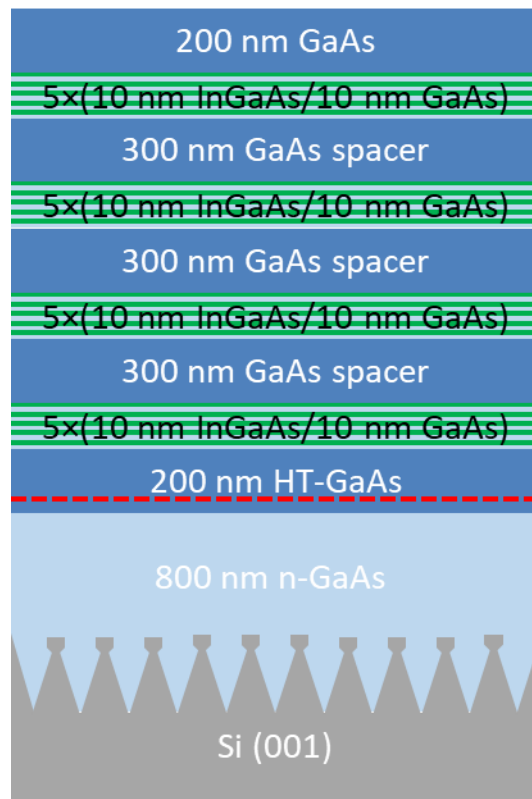
Figure 4.7. Schematic illustration of the whole layer stack of the GoVS.
