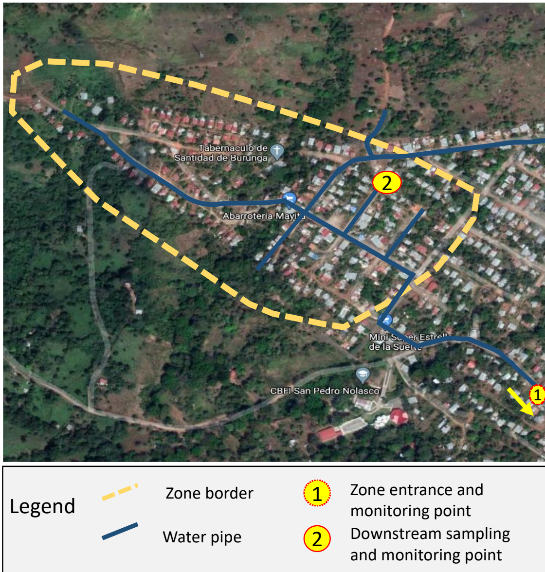
Figure 4.1: Schematic of the IWS zone located in Arraiján, Panama. This zone, with 232 buildings, was supplied water by a pump station managed by IDAAN with a supply schedule that consisted of the provision of water for 3 days followed by 3 days with no supply. This schedule was carried out by IDAAN by manually opening and closing a control valve at the entrance of the area. Because the zone’s entrance monitoring station (with online sensors) experienced frequent negative pressures, grab samples for water quality analysis were collected at the nearby pump station (not shown).
