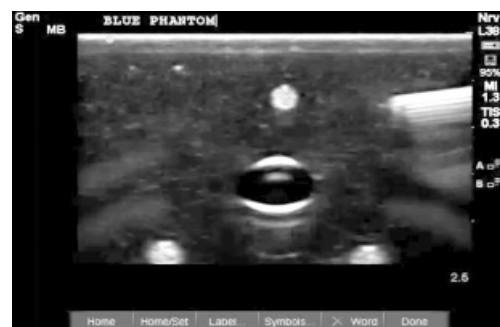
Figure 1. Ultrasound image showing the Blue Phantom model with simulated vascular structure and surrounding nerves.
