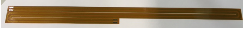
Figure 4.13: Picture of a Simons Array NbTi readout cryocable used to connect the SQUID array amplifiers at T \approx 4 K to the detectors and LC resonators at T \approx 0.3 K. The pairs of NbTi traces are visible through the polyimide insulation and also directly through the exposed connectorization windows at either end. Image courtesy of Masaya Hasegawa.
