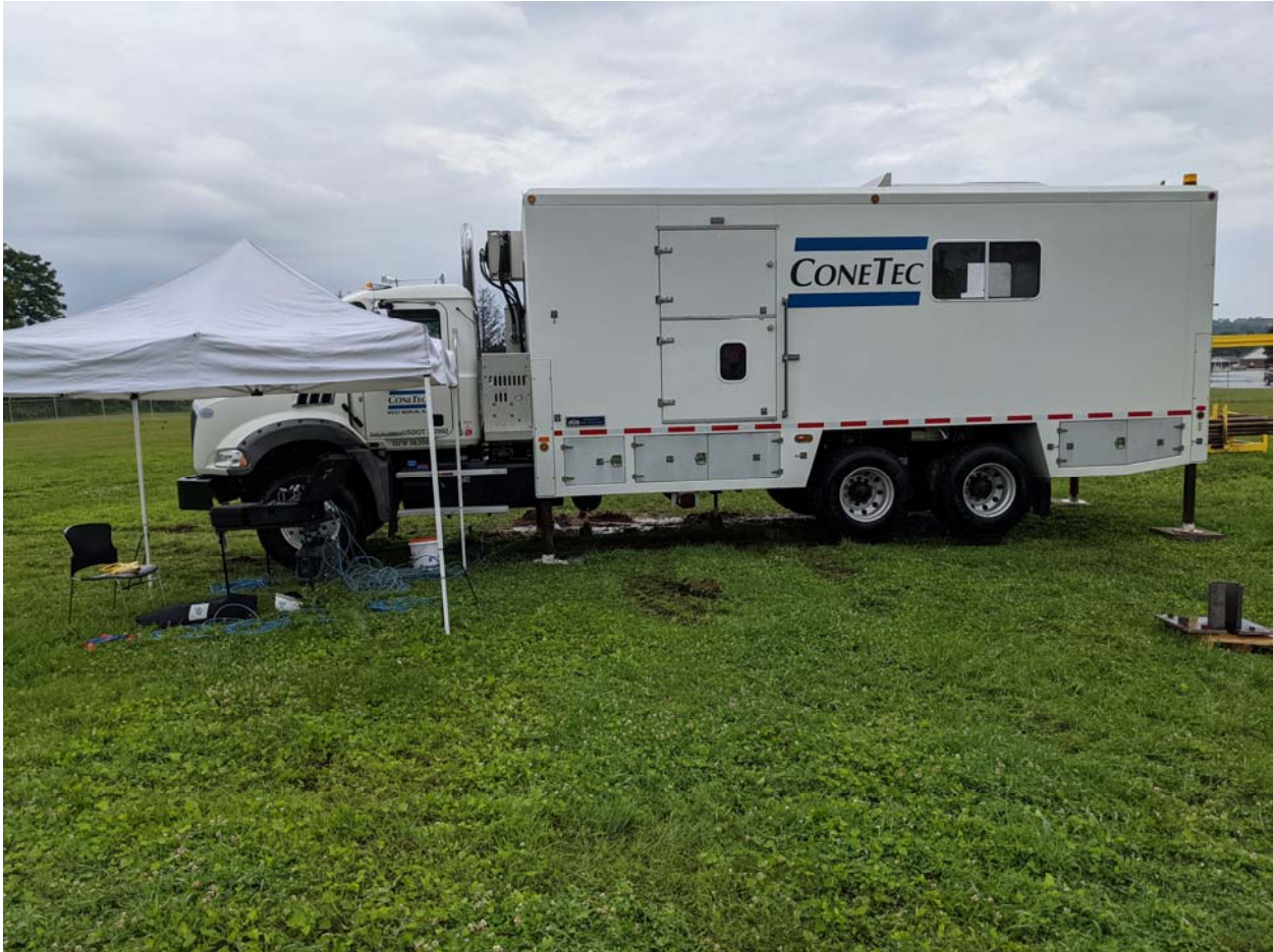
Figure 18 – CPT truck set up over a cased sonic borehole pushing a post-sonic CPT.
