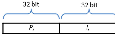
Fig. 10 We reduced the matrix profile to 32 bits and then combined each matrix profile entry and its corresponding matrix profile index entry into a double-precision value to allow fast atomic updates
