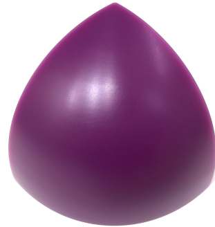
Figure 10: The finished scaled-rotation swept surface with a very fine scallop height of 0.00005 inch, as machined in aluminum 6061 (left) and wax (right).
