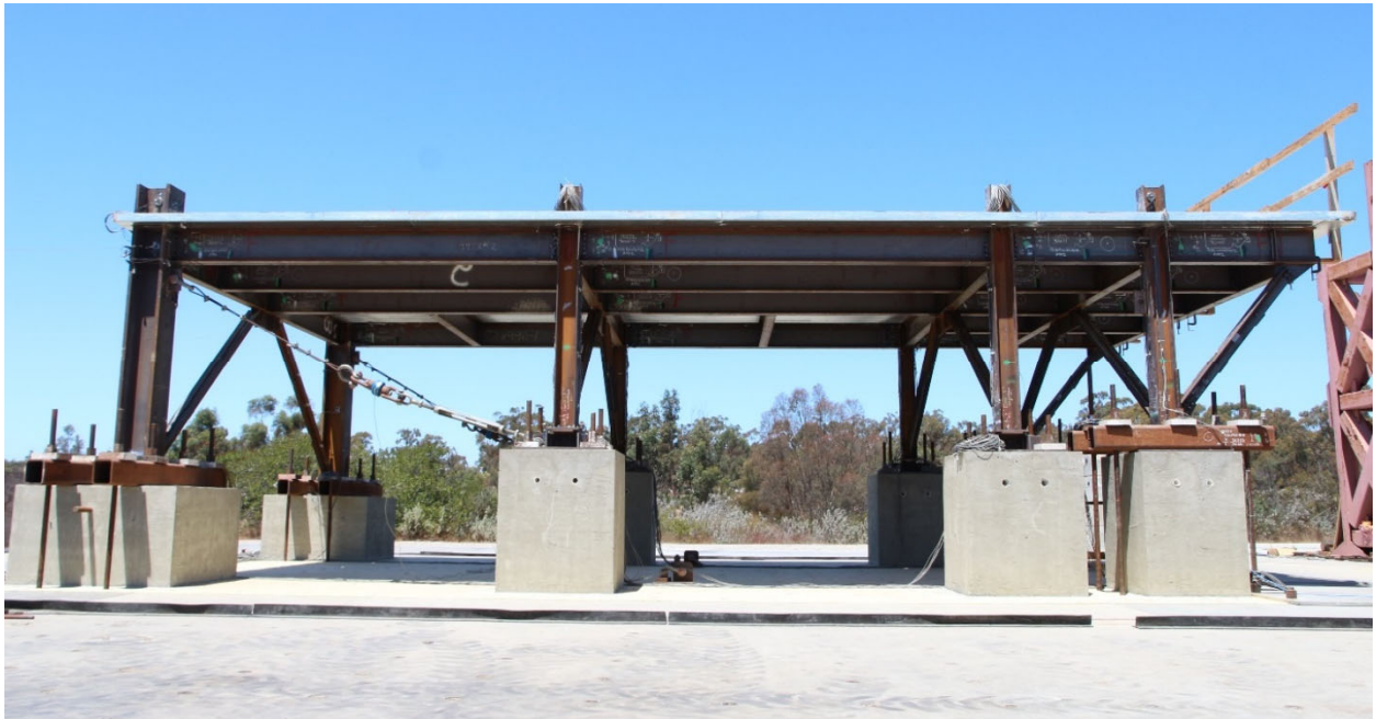
Figure 3.10 Phase 1 Test Building (without Added Mass) Assembled on Shake Table
