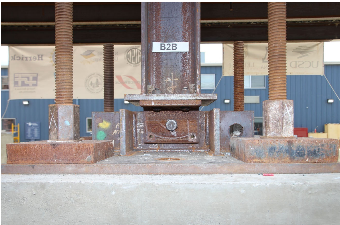
Figure 3.14 Pin-support for Gravity Column
