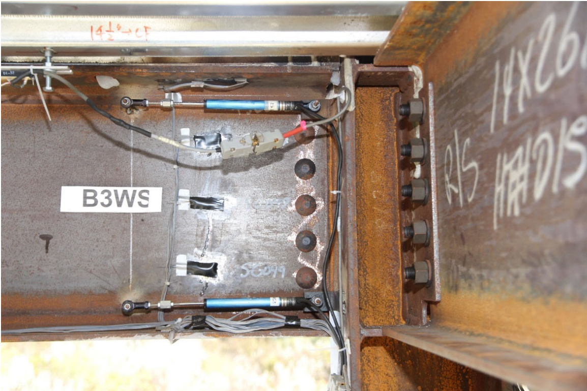
Figure 3.37 Displacement Transducers Installed at Steel Collector-to-Column Connection
