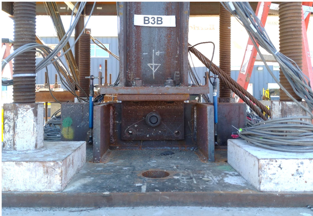
Figure 3.39 Displacement Transducers Installed at Gravity Column Pin-support
