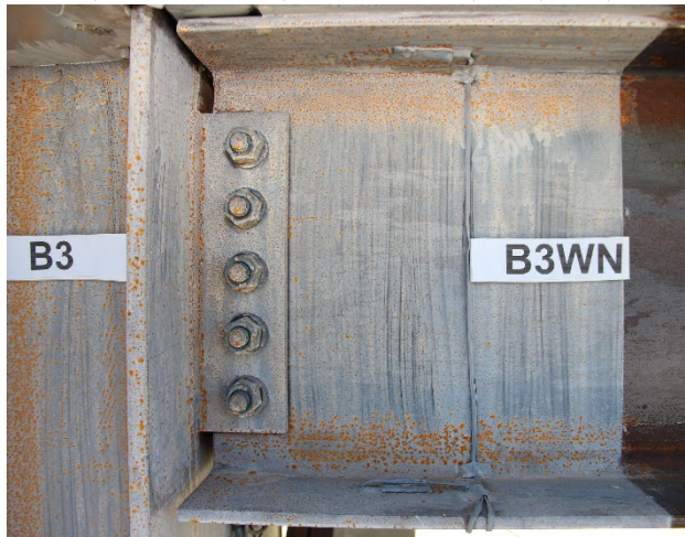
Figure 7.39 After Test 2B-5: Bolt Slippage at 2 nd Floor West-Side BW Connections
