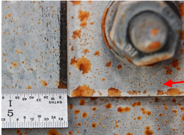
Figure 7.37 After Test 2B-5: Bolt Slippage at 2 nd Floor West-Side TFW Connections
