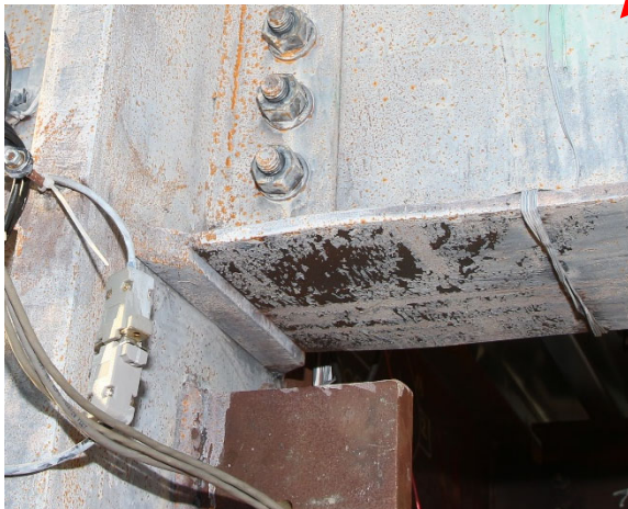
Figure 7.35 After Test 2B-5: Yielding and Local Buckling of Bottom Flange at 2 nd Floor AFW Connection in South Frame
