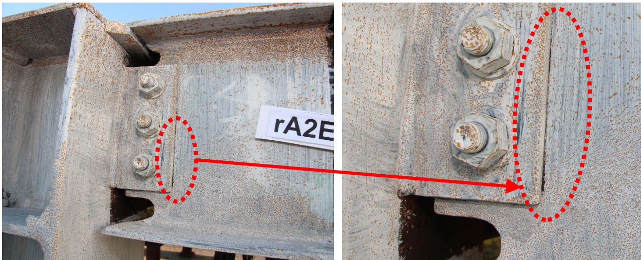
Figure 7.25 After Test 2B-3: Bolt Slippage at Roof East-Side TFW Connections
