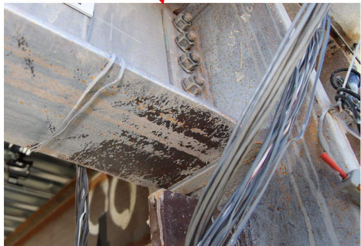
Figure 7.36 After Test 2B-5: Yielding and Local Buckling of Bottom Flange at 2 nd Floor AFW Connection in North Frame
