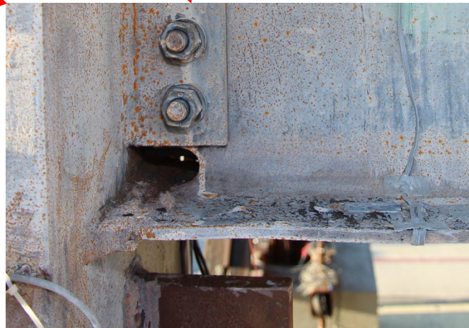
Figure 7.35 After Test 2B-5: Yielding and Local Buckling of Bottom Flange at 2 nd Floor AFW Connection in South Frame
