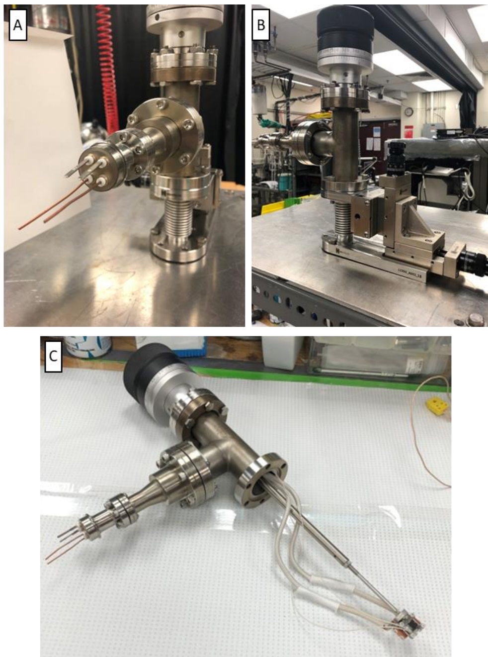
Figure A.3: (A) Side view of the set up with the copper heating rods and thermocouple attachments. (B) View of the components outside the vacuum chamber with the manipulator, T-shaped attachment and the rotary manipulator. (C) Full set up of the T-shaped attachment and rotary arm with block and heating and thermocouple wires attached.
