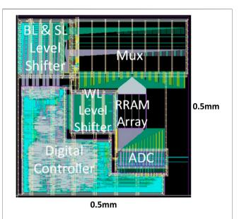
FIGURE 7 | CIM macro layout implemented with TSMC 40 nm RRAM process.
